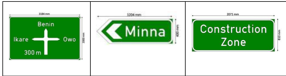
Figure 5.16: Typical Information Sign Designs using Trafsoft
